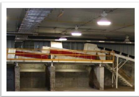
**REFINING AND STORAGE.** Compost is moved from Phase 2 Curing to the Storage area where the compost is screened and stored until shipped. The screening operation separates the compost into 3 size categories; 75 percent compost (less than 12mm); 20 percent mulch (12mm to 30mm) and 5 percent oversize. The compost and mulch fractions are suitable for sale as soil conditioner, or can be recycled through the process as amendment. The oversize material is sent to landfill.
