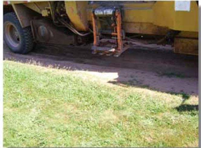
Potholes can cause damage to the low mounted cart flipper.
